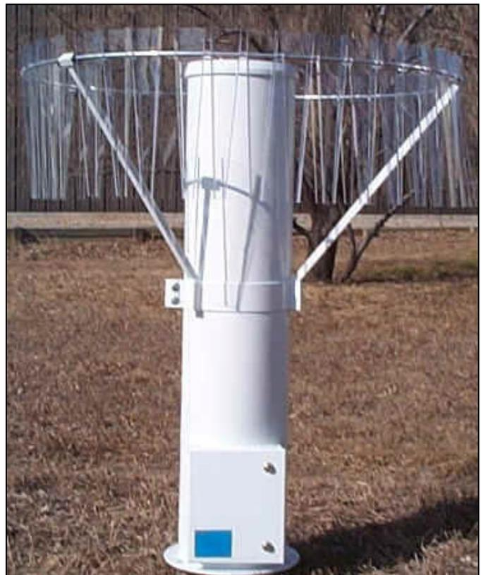
MODEL 5045-30 All Weather Rain Gauge with 30 inch Capacity and optional wind screen.
